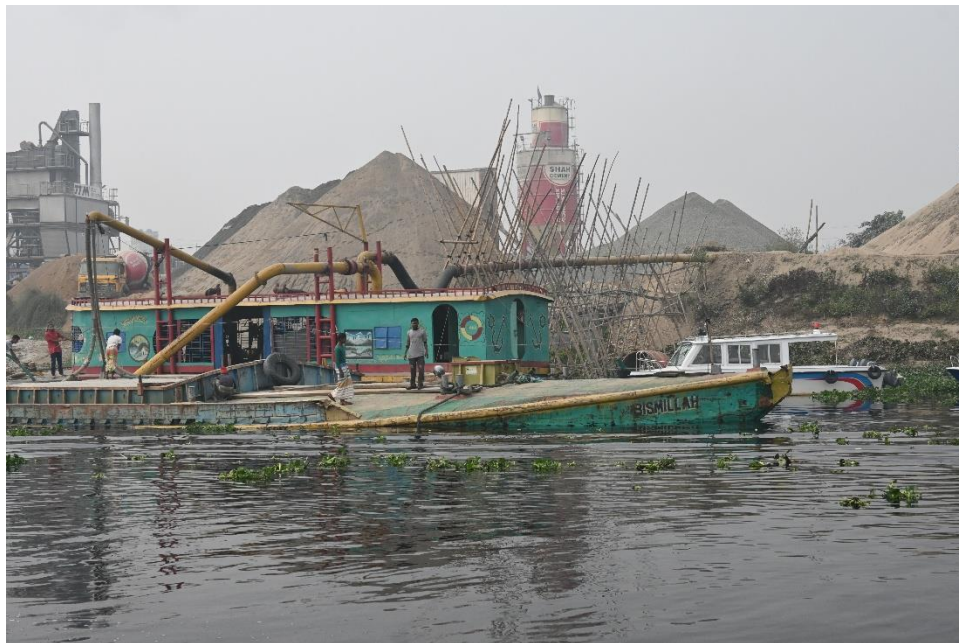
Figure 7: A dredging boat pumping sand into a landfill site [15].
